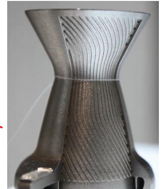
L-PBF Cooling channel example
